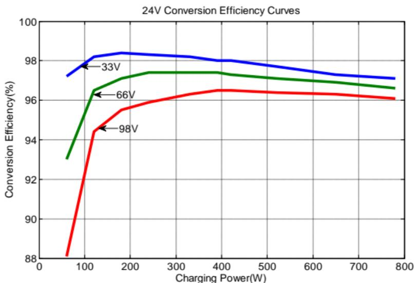
Tracer4215BN Illumination Intensity: 1000W/ m<sup>2</sup> Temp: 25 °C
