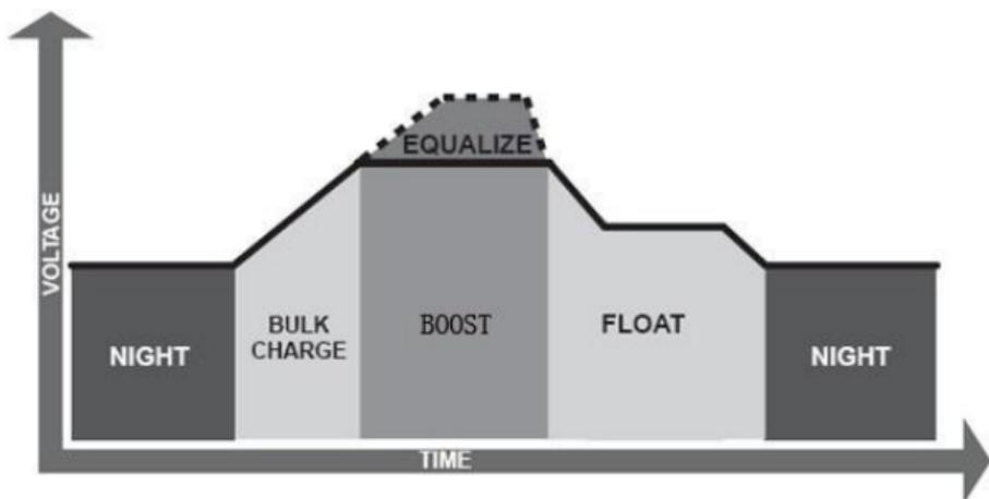
Figure 4-2 Tracer-BN series MPPT charging algorithm
