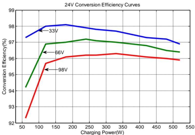
**Tracer3215BN**    **Illumination Intensity: 1000W/ m<sup>2</sup>**    **Temp: 25 °C**
